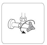
10. Turn on the knob to check whether the nozzle is protruding;
